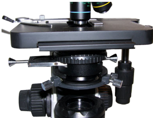
Condenser NA 0.9 with phase slider inserted.
